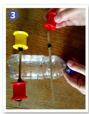
Push the bobbins onto the end of the axles. Use elastic bands to hold them in place.
